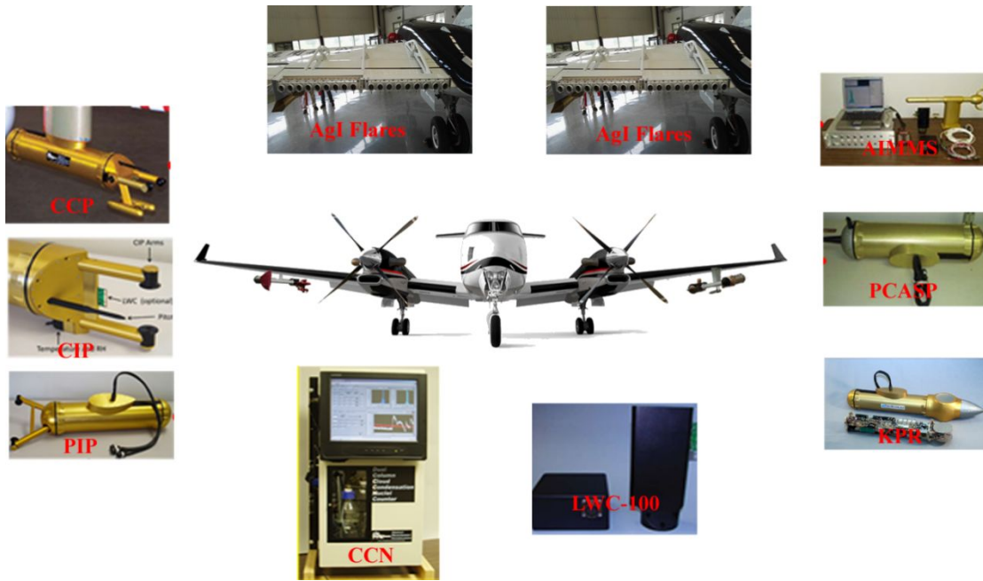
695 Figure 1. Photos of the KingAir aircraft probes, including AgI flares equipment, Ka-band 696 cloud radar (KPR), cloud combination probe (CCP), cloud imaging probe (CIP), precipitation 697 image probe (PIP), 20 Hz Aircraft-Integrated Meteorological Measurement System 698 (AIMMS-20), Passive Cavity Aerosol Spectrometer Probe (PCASP), cloud condensation 699 nuclei (CCN) counter and Hot-Wire Liquid Water Content Sensor (LWC-100).
