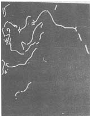
Fig.5. Edges from Fig. 4 after cleaning / semi-pixel thickening / thinning.
