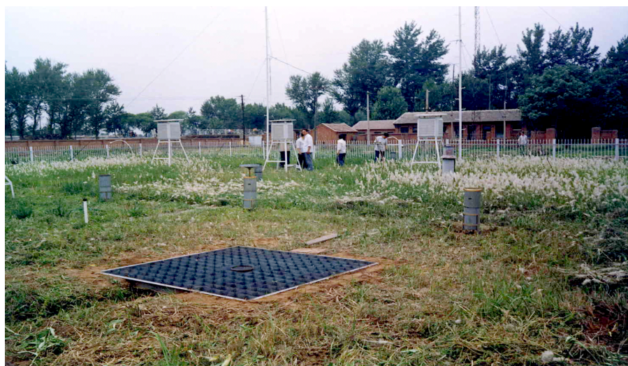
Fig. 3. Picture of an evaluation station. Note that there are two operational gauges located at two sides of the horizontal gauge in the middle part of the picture and a pit gauge at the surface in front of them.
