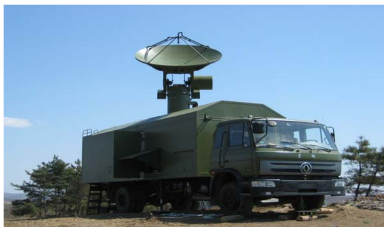
Fig. 10. X-band polarization Doppler radar in Institute of Atmospheric Physics, Chinese Academy of Sciences.
