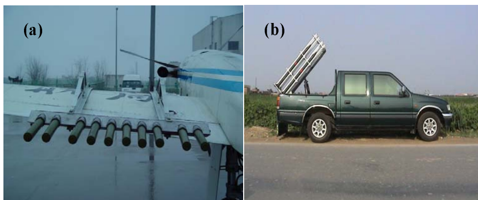
Fig. 11. Seeding tools widely used in current weather modification operation in China, (a) aircraft seeding system equipped with AgI flare agent, (b) mobile AgI-rocket launching system.
