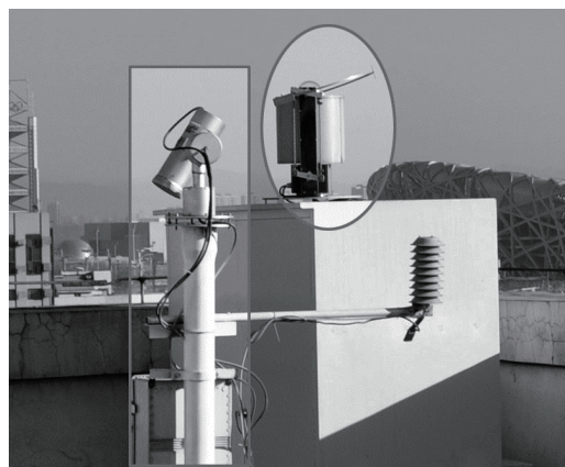
Fig. 1. The ASI (circled) and SIRIS (highlighted in a rectangle) located on the office building of the Institute of Atmospheric Physics, Chinese Academy of Sciences.
