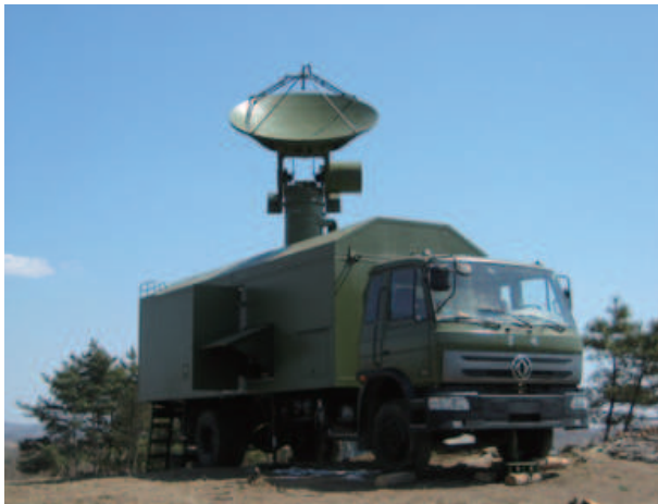
Fig. 6. X-band polarization Doppler radar used in field experiments operated by the Institute of Atmospheric Physics, Chinese Academy of Sciences.
