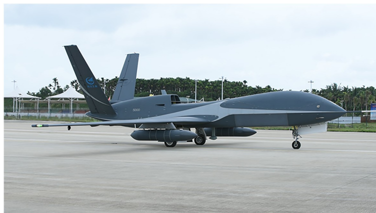
Fig. 2. The Yilong-10 UAV used in the experiment (Carried underneath the wings of the UAV are the dropsonde systems.).
