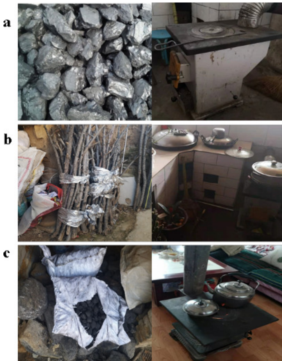
Fig. S1. Common domestic solid fuels and stoves in Tongchuan of the Fenwei Plain in China (a: lump coal, b: biomass, and c: clean coal).
